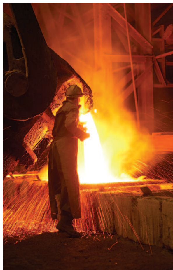
Pouring copper in the Tsumeb smelter.
